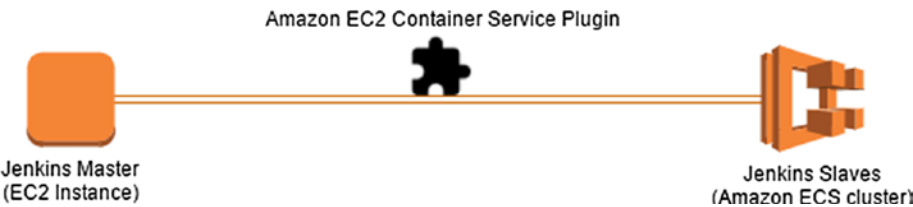
Figure 4-10. Scalable Jenkins Slave cluster using ECS Instances
