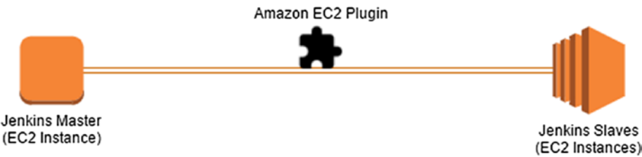
Figure 4-9. Scalable Jenkins Slave cluster using EC2 Instances
