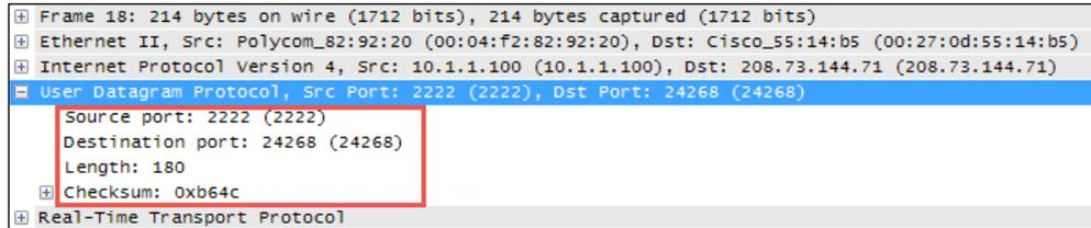
The UDP header is only 8-bytes long, consisting of:
