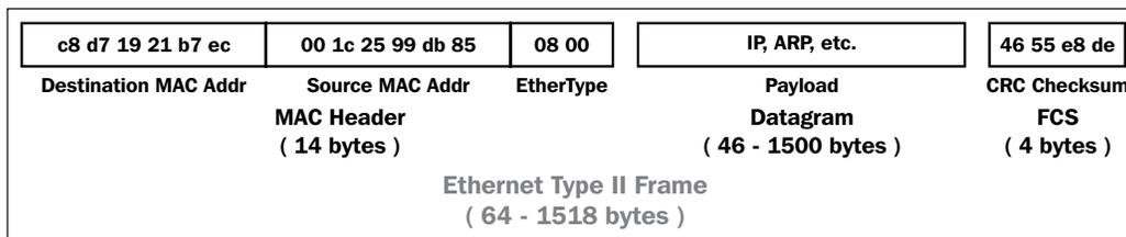
A key point here—and this is important to understand—is that Ethernet frames and their MAC addresses are only able to transmit frames between devices on the local area network (LAN and IP subnet) they belong to.
