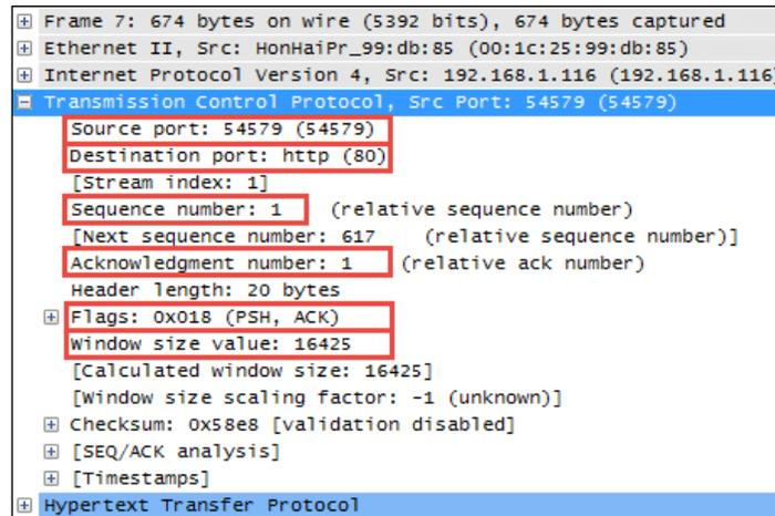
The TCP header contents and length can vary depending on options that may be in use, but in its simplest implementation it consists of:
