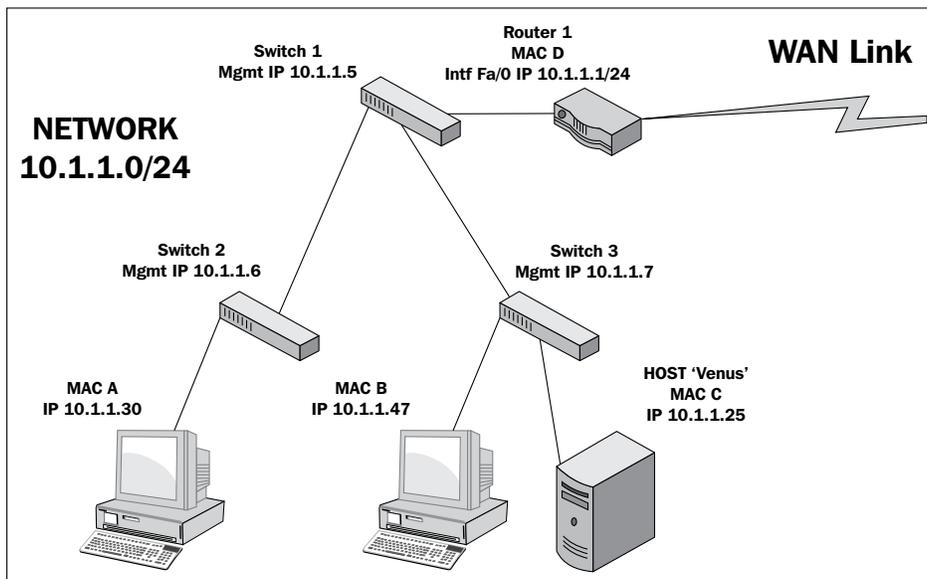
The following two scenarios leverage this drawing to show how MAC addresses are utilized to switch Ethernet frames around local area networks:
